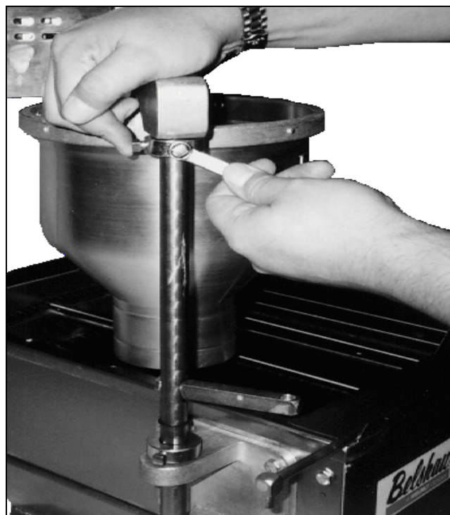
Figure 1-9. Adjusting the Swing of the Hopper.
