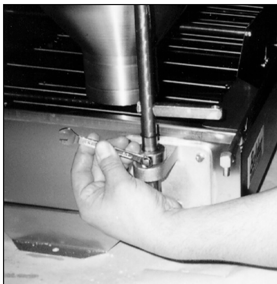
Figure 1-8. Adjusting the Height of the Hopper.
