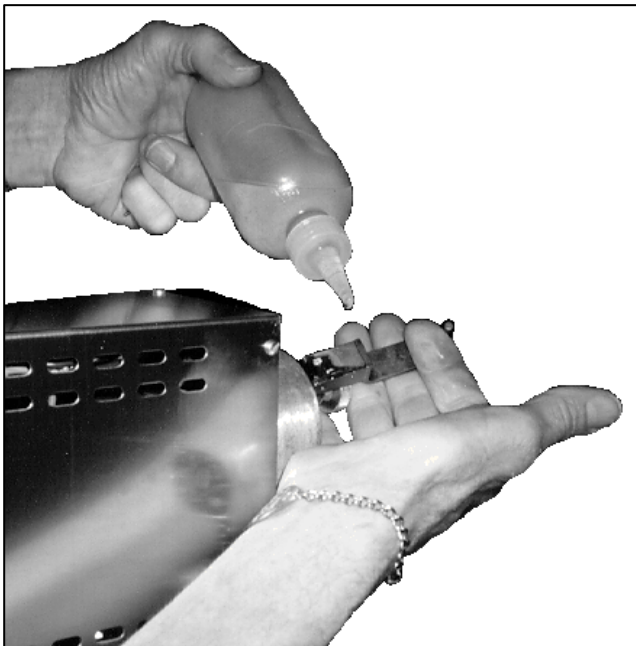
Figure 3-1. Lubricating the Connecting Rod Assembly.
