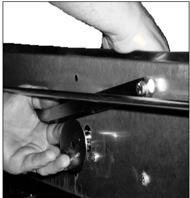
Figure 2-2. Removing the Turner Cam Assembly.
