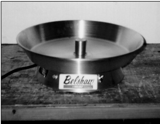
Figure 4-4. Sugaring Tray and Roto Cooler.
