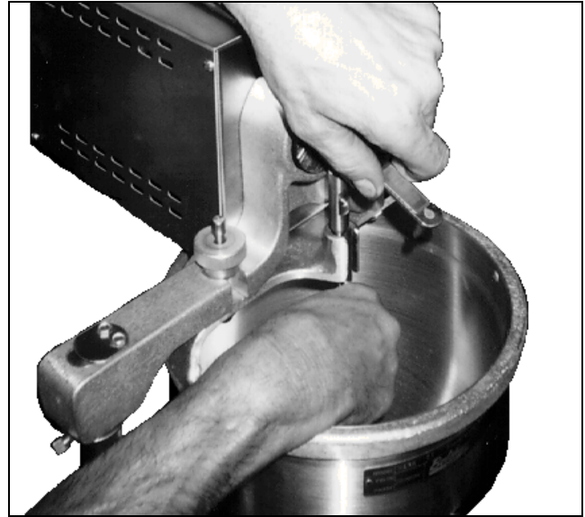
Figure 1-7. Installing the Plunger.
