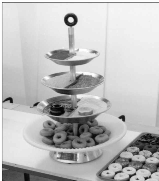
Figure 4-3. Icing Finishing Tree with Roto Cooler.
