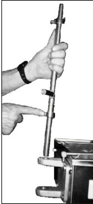
Figure 1-3. Inserting the Swing Column.
