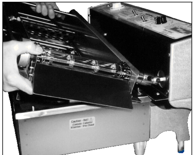
Figure 1-2. Joining the Couplings.
