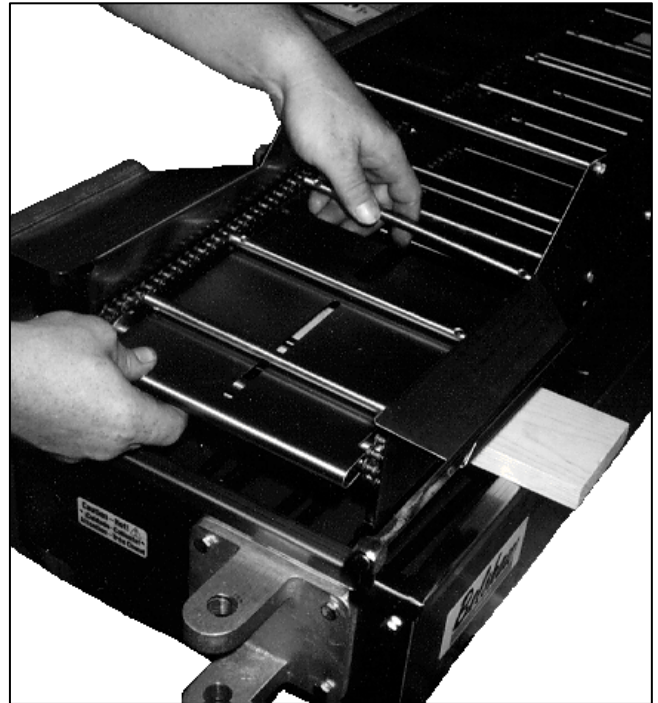
Figure 2-4. Removing the Drop Plate.
