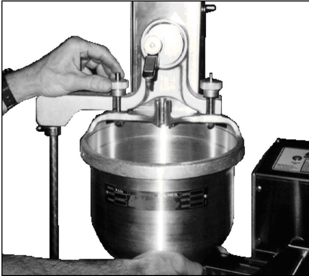
Figure 1-6. Mounting the Hopper.
