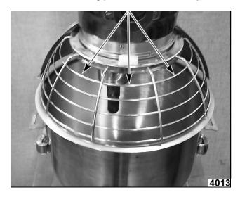
2. Insert the chute between the second and third wires being sure to engage chute hooks on top wire.
