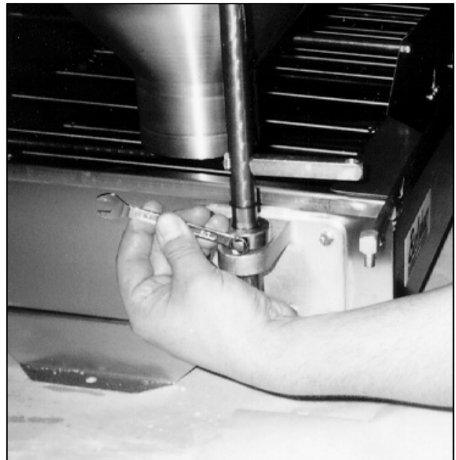
Figure 1-10. Adjusting the Height of the Hopper.
