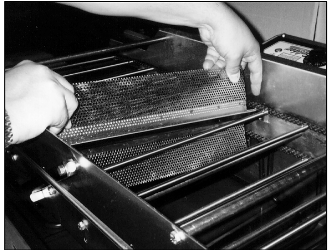
Figure 2-3. Removing the Turner Cam Assembly.
