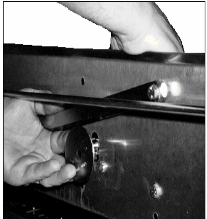
Figure 2-4. Removing the Turner Assembly.
