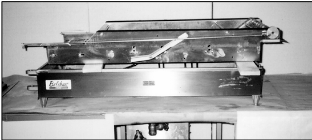
Figure 2-2. Draining the Shortening off of the Conveyor.
