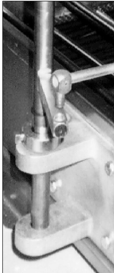
Figure 1-6. Connecting the Swing Connecting Rod.
