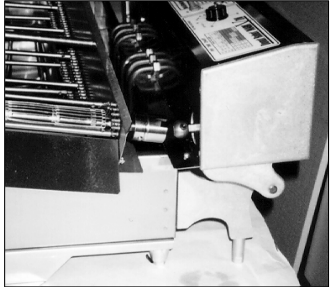
Figure 1-3. Joining the Couplings.
