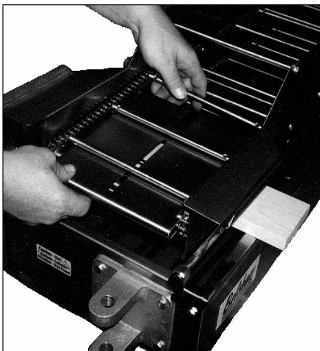
Figure 2-5. Removing the Drop Plate.
