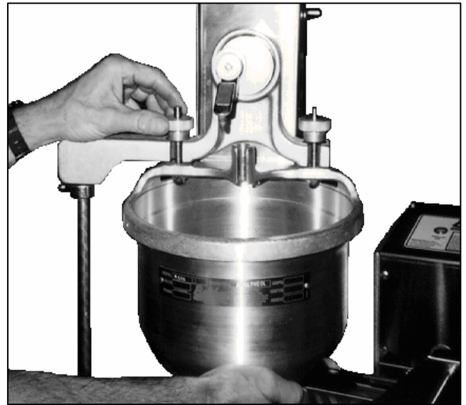
Figure 1-8. Mounting the Hopper.
