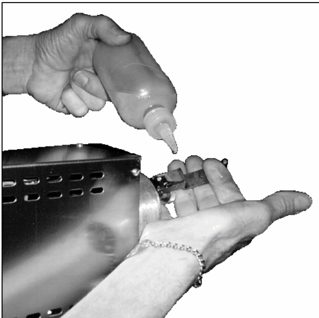
Figure 3-1. Lubricating the Connecting Rod Assembly.
