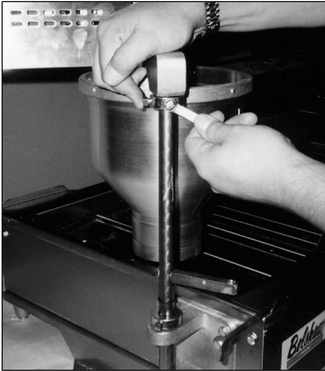
Figure 1-11. Adjusting the Swing of the Hopper.
