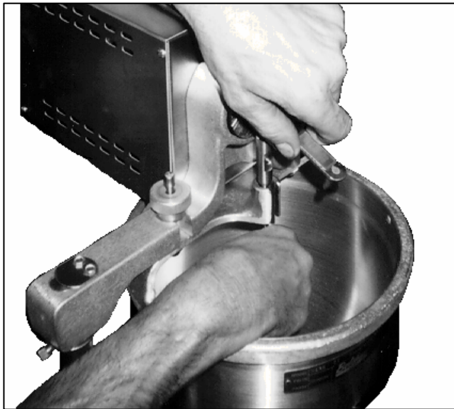
Figure 1-9. Installing the Plunger.
