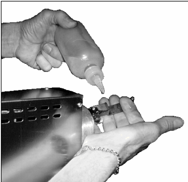
Figure 2-1. Lubricating the Connecting Rod Assembly.
